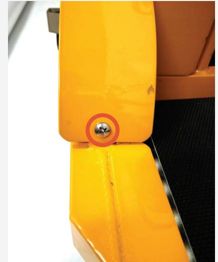
Image 2: Screw on protective cover, side.
