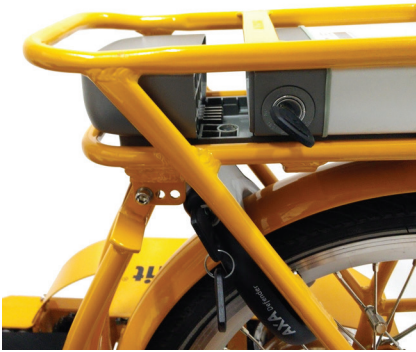
Image 7: Press and turn the key counterclockwise to remove the battery.
