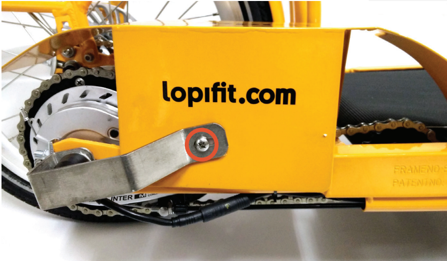
Image 1: Screw on protective cover, front.
