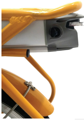
Image 8: Plug connector, pull the tab towards you.
