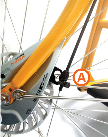
Image 12: Front brake disengagement point A.
