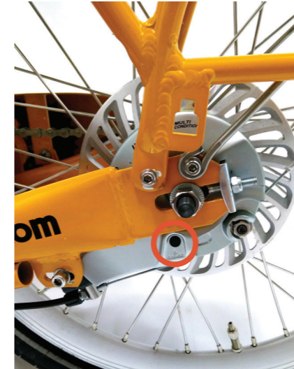
Image 17: Remove the brake cap and add brake grease.
