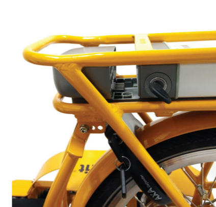
Image 7: Press and turn the key counterclockwise to remove the battery.
