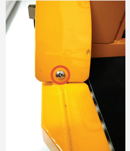
Image 2: Screw on protective cover, side.
