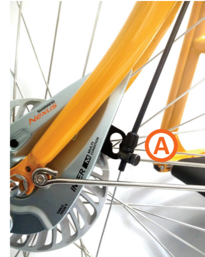
Image 12: Front brake disengagement point A.
