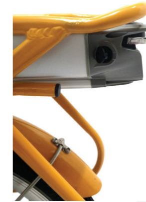
Image 8: Plug connector, pull the tab towards you.
