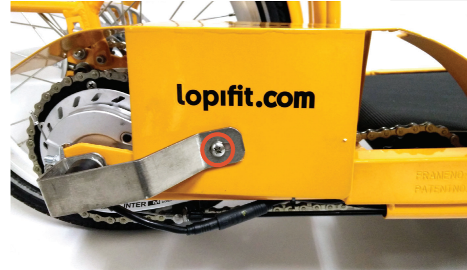
Image 1: Screw on protective cover, front.
