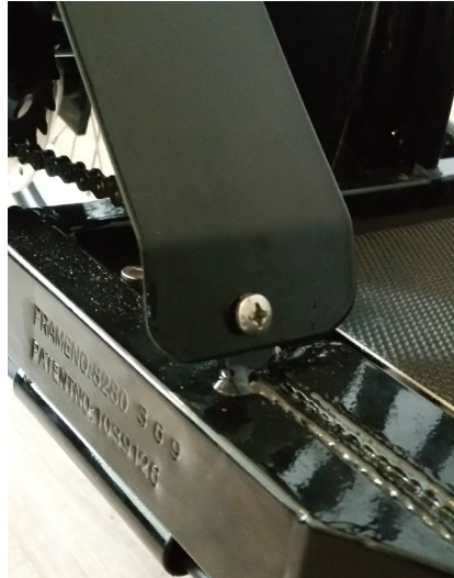
Image 2: Screw on protection cap, side.
