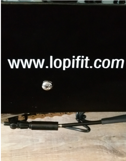
Image 1: Screw on protection cap, front.
