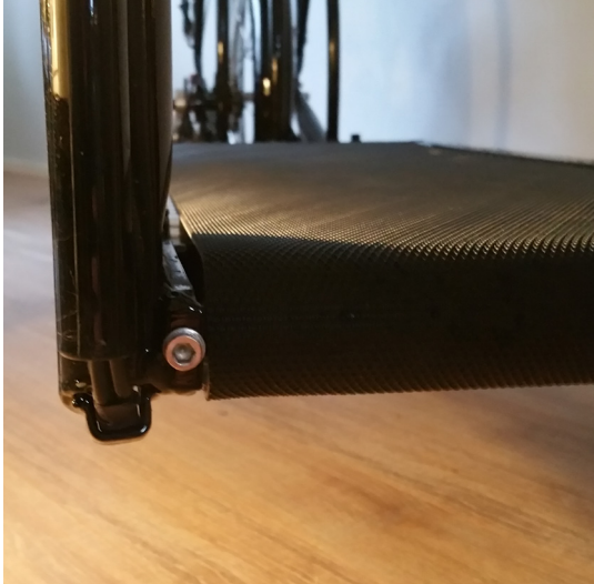
Image 7: Tension adjustment bolt, left.
