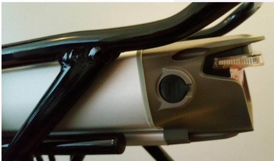
Image 12: Charge socket, pull the tab.
