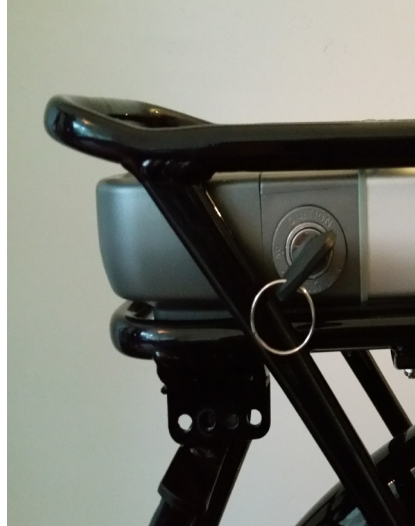
Image 10: Key vertical, battery is off.
