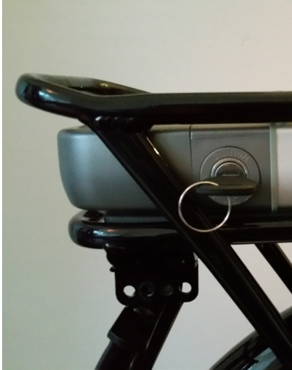
Image 9: Key horizontal, battery is on.
